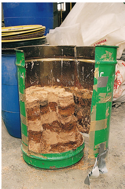
Fig. 4. Soil–grout columns during extrusion.
